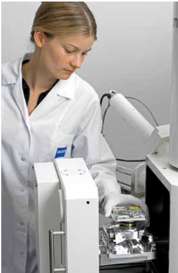
Shuttle & Find being used in the specimen area of an electron microscope.
