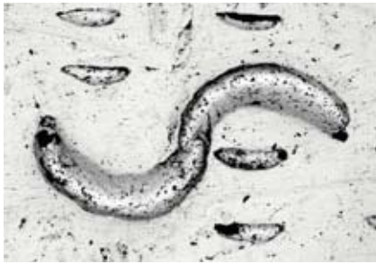
The goldsmith positioned the half-moon shaped tool several times to create an S-shaped structure.
