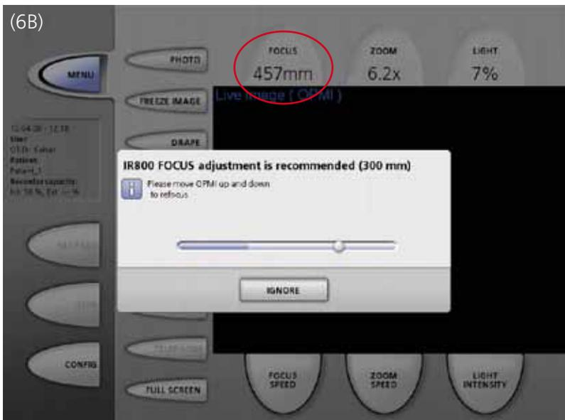
**Fig. 6B:** A message is displayed when the actual focus (in this case 457mm) exceeds the recommended focus distance (less than 300mm). In this case the microscope should be brought closer to the surgical field.
