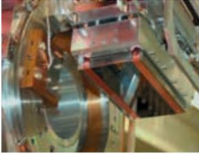
The picture is courtesy of GKSS, Incoatec and Prof. Stamparoni/SLS and shows a 2 stripe coated mirror with a Ru/C and W/Si multilayer coating mounted in the monochromator of the TOMCAT beamline at the SLS.
