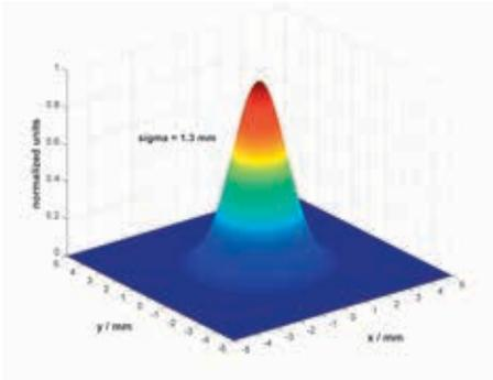
*Gaussian type removal function typical of CCP or IBF.*
