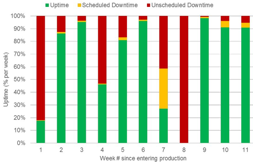
**Figure 5:** Tool availability recording. The different columns represent the weeks for which uptime has been recorded by Intel after tool insertion into production. The categorization Uptime-Downtime is shown in color code, in which a full week time is set to 100%.
