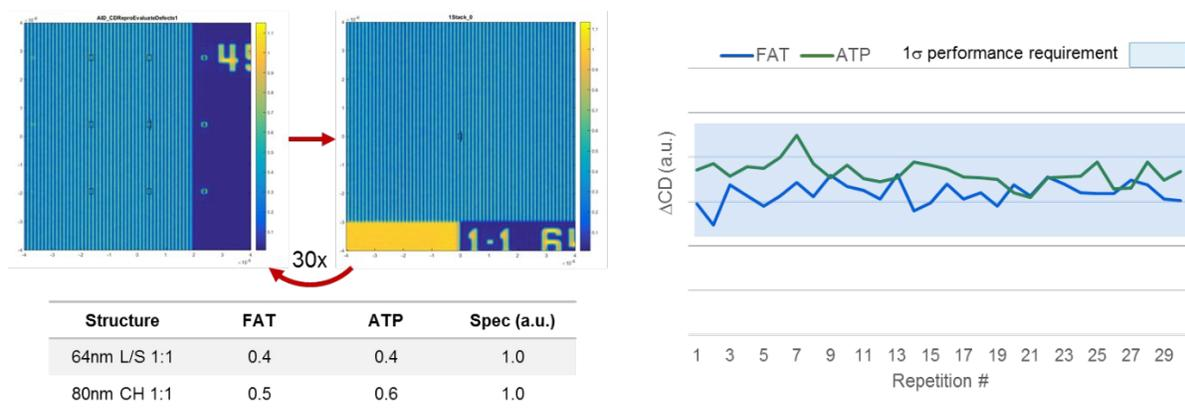
**Figure 3:** Top left: Exemplary defect and reference images of a lines and spaces dense array used for qualification of CD reproducibility measurements. Right:  $\Delta\text{CD}$  values measured for the central defect ROI at factory and final acceptance, in which the blue area represents a  $1\sigma$  performance requirement. Bottom left: CD reproducibility results at factory (FAT) and final acceptance (ATP) normalized to a specification value of 1.0.
