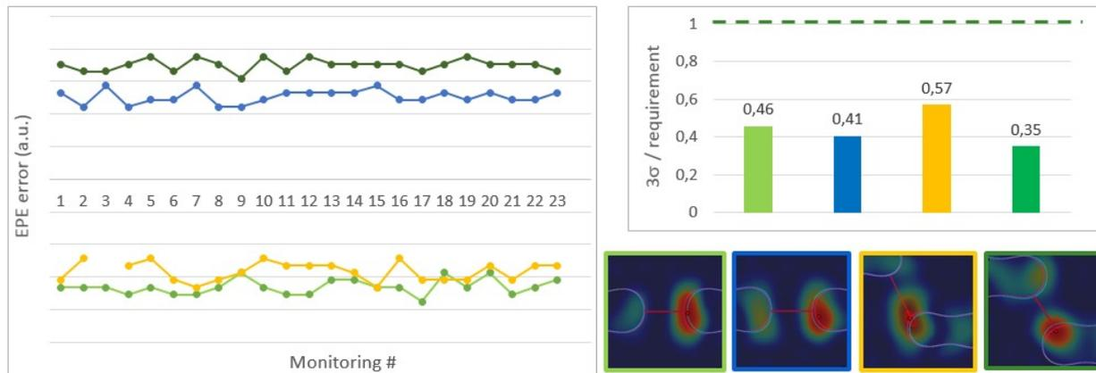
**Figure 10.** Left: Results of the EPE measurement stability monitoring, reported in arbitrary units. The four series shown in the plot refer to the four different defects analyzed by the monitoring, displayed at the bottom right with color coded frames. Right: statistical analysis of the EPE measurements for the four defects. The values reported are  $3\sigma$  normalized to the budget requirement.
