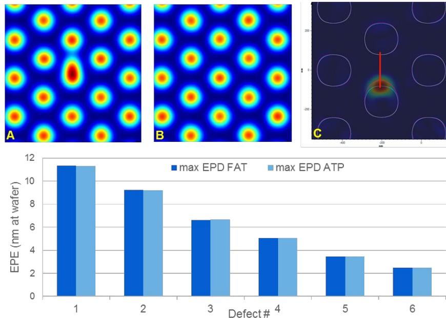
**Figure 4:** Top: aerial image of the staggered contact holes used for EPE measurement during factory and final acceptance. A. Defect image. B. Reference image. C. Reference and defect image contours superimposed to the defect – reference difference aerial image. The slice used for CD measurement is displayed as a red line connecting two adjacent contours.
