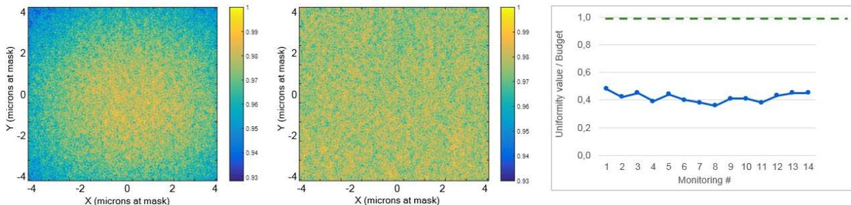
**Figure 7:** Description and monitoring result of the AIMS™ EUV field illumination uniformity. Left: raw aerial image of a clear field on a EUV mask as acquired by AIMS™ EUV (see text for features description). Center: clear normalized aerial image of the same mask reflective field. Right: Field illumination uniformity for all monitoring occurrences, values are normalized by the budget requirement.
