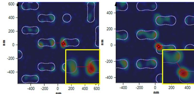
**Figure 9:** Defect – Reference difference aerial image and contours of two defect types used for AIMS™ EUV EPE measurement stability monitoring in Intel mask shop. The red cross highlights the defect center, whereas the defective area is displayed within the central area. Within the yellow frame, a zoom in the defective region is displayed.
