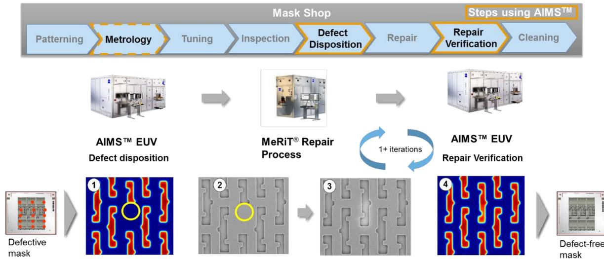
**Figure 1:** Exemplary mask production flow process. On the top line and in orange highlighted, the steps in which AIMS™ EUV is used. Bottom panel: 1. AIMS™ EUV aerial image of the defect. 2. Mask SEM image of the defective area acquired by the MeRiT® before repair. 3. Mask SEM image of the repaired area. 4. AIMS™ EUV aerial image of the repaired defect.
