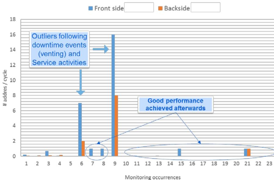
**Figure 6:** Particle contamination monitoring results. The number of adders per cycle is plotted in blue and orange for the mask front and back side respectively. Monitoring runs contain different number of cycles.
