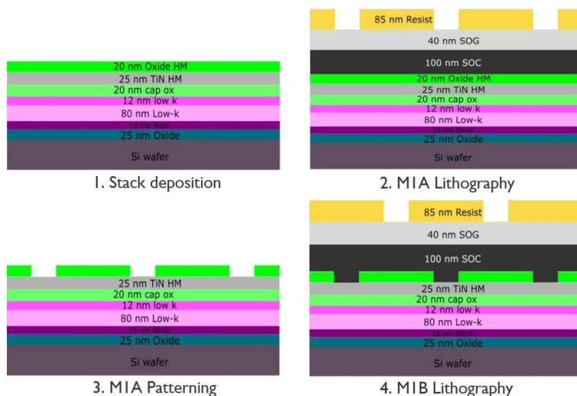
Figure 6. Schematic representation of the lithography process flow.
