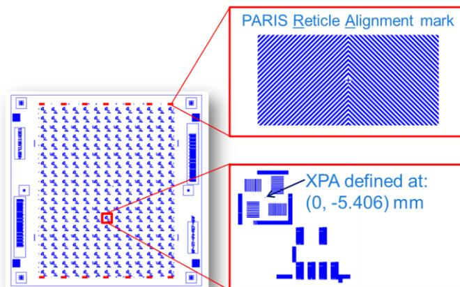
Figure 2: Layout of the mask that was used in this experiment. The image field contains metrology modules in a  $13 \times 19$  layout. Each module contains an XPA wafer alignment mark that can be read by the scanner alignment sensor. PARIS reticle alignment marks ( $2 \times 7$ ) at both ends of the mask were used to align the reticle.
