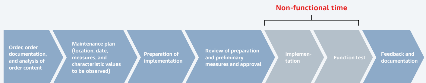
Figure 7: General phases of repair
